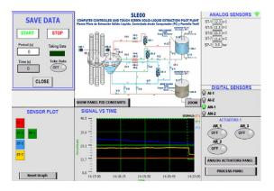
Real time representation of any measured variable of the SLEOO pilot plant.
