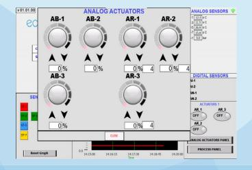
The SLEOO pilot plant allows manual control of the process flow rate and the performance of the heating
